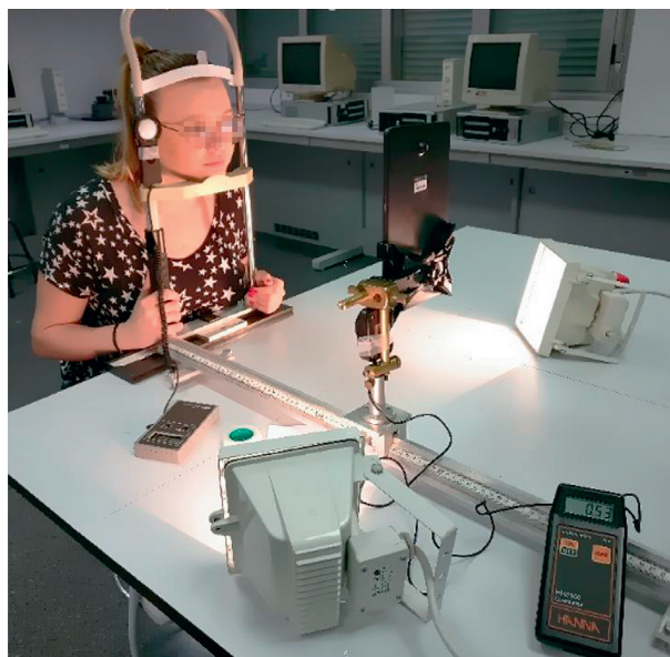
FIGURE 4: Laboratory setup for evaluating accuracy of illumination measurements. Face position was fixed with a chin and forehead rest. A lux meter was placed temporal to the right eye and in the eye plane.
