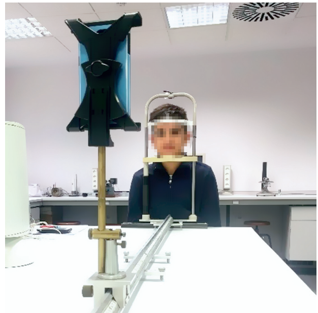
FIGURE 2: Laboratory setup used for testing the accuracy of face-device distance measurements. Face position was stabilized with a chin and forehead rest, and the mobile device position was adjusted along the optical bench.
