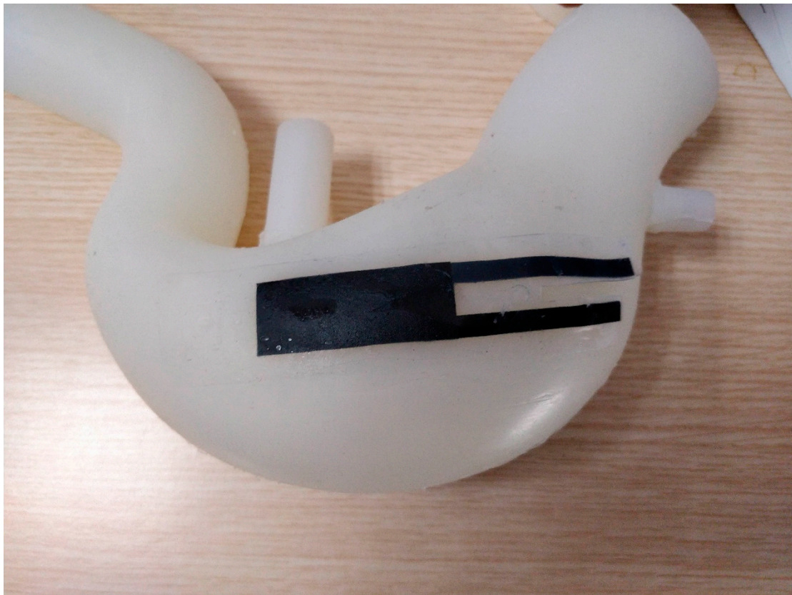
Figure A2. Placement of sensor on silicone in vitro stomach model—anterior wall of body.
