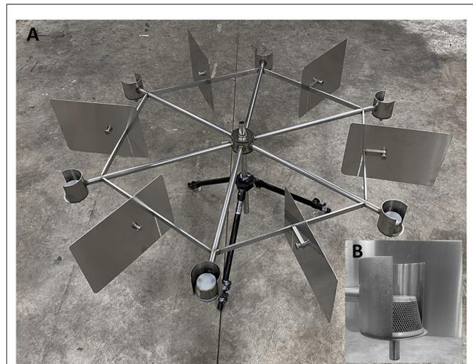
**FIGURE 1** | Testing Wheel Image: **(A)** Stainless-steel testing wheel with 6 radial arms and sample divider plates between positions; **(B)** Walled (3/4 circumference) cups and wire basket for sample presentation.
