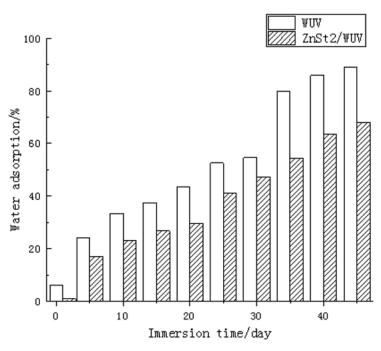
Figure 5. Water resistance test of WUV and ZnSt2/WUV.
