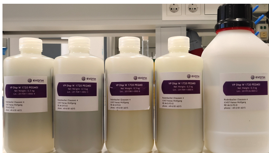
Figure 2. Concentrated solutions of hydrophilic silica nanoparticles as received from Evonik Industries; from left to the right: NF1, NF2, NF3, NF4 and NF5.
