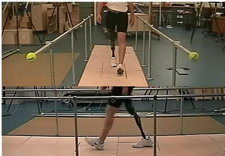
**Fig 1. One trans-femoral amputee subject walking on the 2.5° camber walkway.**
