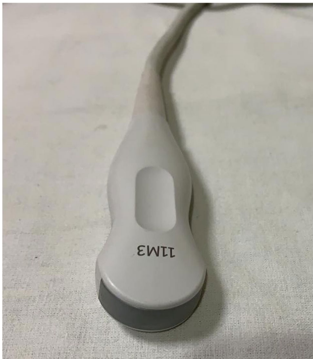
Fig. 2 Micro-convex array ultrasound transducer with frequency of 4 to 10 MHz, indicated for pediatric use as it has a small footprint
