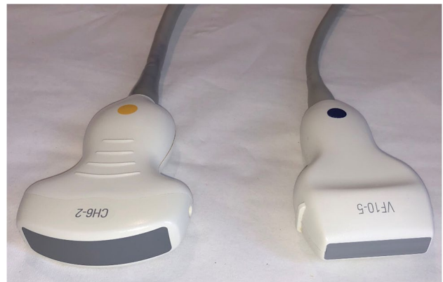
Fig. 3 Convex and linear transducer. Left image: convex transducer with frequency of 3 to 5 MHz. They have a curved array that allows wider field of view. These are used for abdominal scans and have deeper penetration due to low frequency. Right image: linear transducers have a flat array and appearance. They have high frequency and are useful for small parts and shallow structures near the surface of the body. They produce a rectangular image with frequency ranging from 9 to 14 MHz
