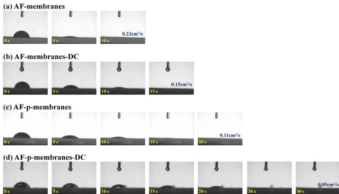
Figure 7. Diffusion rate of a water droplet on the PVDF/CFO membranes: (a) AF-membranes with 0.23 \text{ cm}^2/\text{s} , (b) AF-membranes-DC with 0.15 \text{ cm}^2/\text{s} , (c) AF-p-membranes with 0.11 \text{ cm}^2/\text{s} , and (d) AF-p-membranes-DC with 0.05 \text{ cm}^2/\text{s} .
