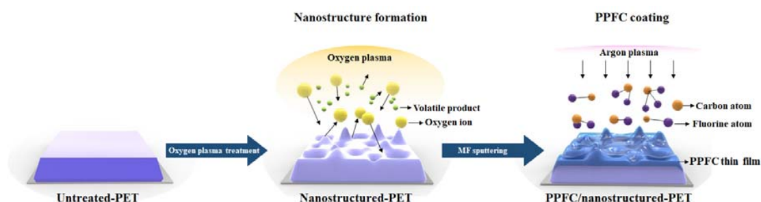
Figure 1. Schematic of the nanostructure formation and plasma-polymer-fluorocarbon (PPFC) thin film coating process.
