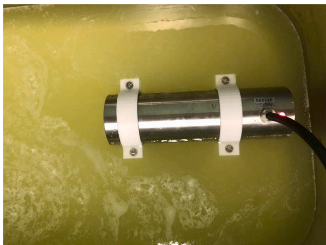
Fig. 1. Laboratory installation for high-intensity (45 KHz) cavitation processing of native milk curd whey.
