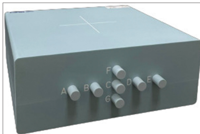
Figure 1: The Mobius Verification Phantom™ with seven slots for insertion of the ionization chamber (A to G location)
