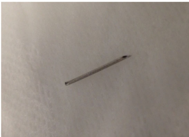
Figure 2: The 15 mm tip of the EBUS-TBNA needle showing the site of fracture close to the junction between the long, shiny electroplated section and the coarse distal end.
