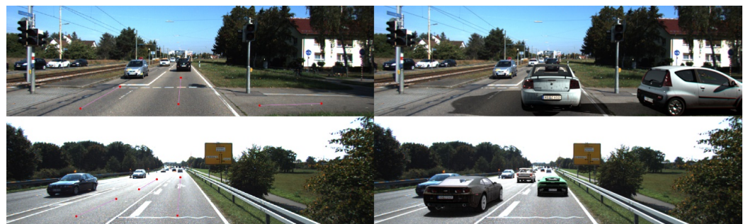
Figure 6. Marking trajectories on the original images (left) and augmenting image by rendered models at random positions on the trajectories (right).
