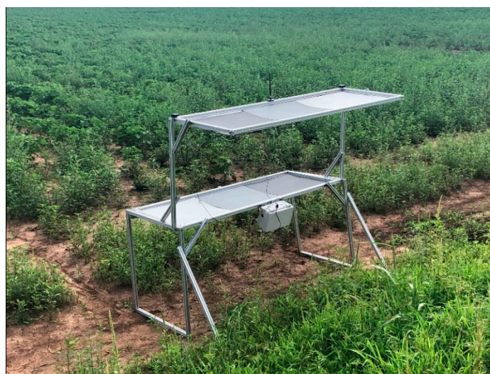
Figure 8. Real constructed multifunctional GCP used for georeferencing, radiometric calibration, and height calibration.
