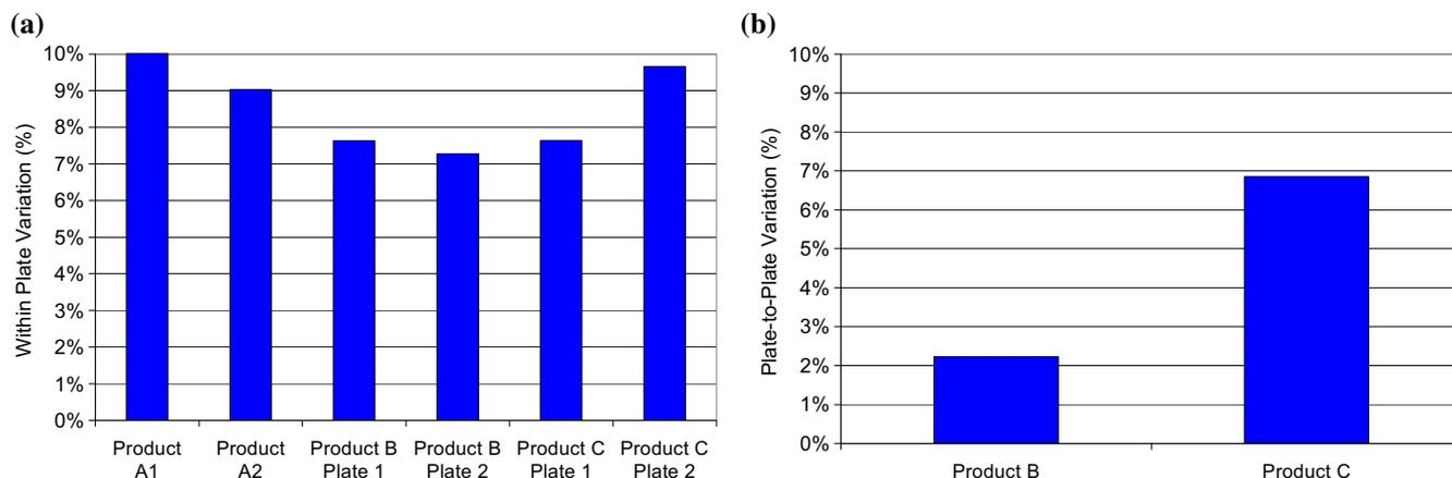
**Figure 10.** (a) Within plate titer variation (one standard deviation) for the Hamilton/96DW process for six plates ( $n = 96$ ). (b) The plate-to-plate variation for monoclonal antibodies B and C ( $n = 192$ ). Titer in diluted culture medium samples was measured using an Octet QK384.
