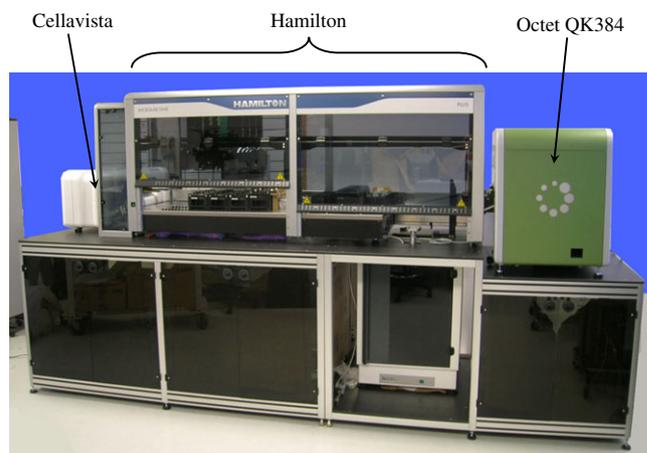
Figure 9. Integrated high throughput screening tool consisting of a Hamilton STARplus liquid handler, Cellavista cell counter, and Octet QK384 protein quantitation tool.
