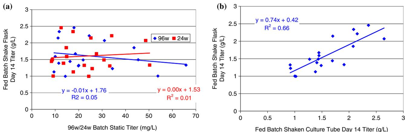
**Figure 2.** (a) Correlation graph of fed-batch shake flask titers with 96w and 24w static batch titers for monoclonal antibody A ( $n = 20$ ). (b) Correlation graph of fed-batch shaken culture tube titers with fed-batch shake flask titers for monoclonal antibody A ( $n = 20$ ).
