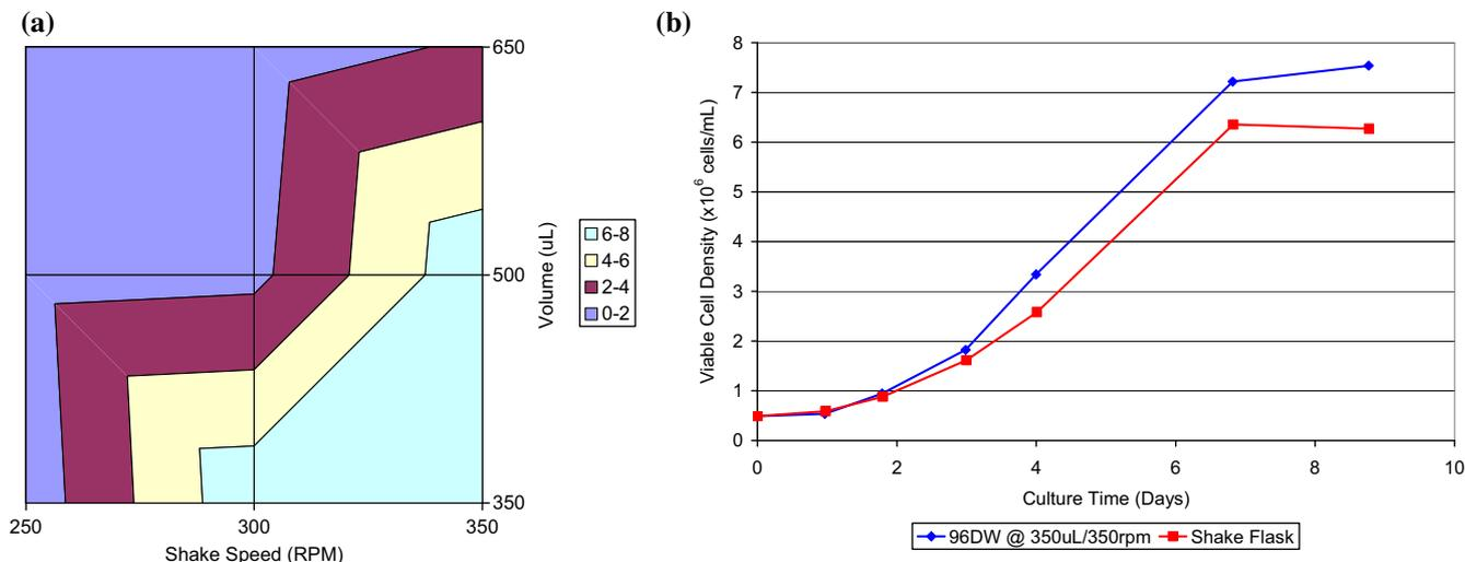
Figure 7. (a) Viable cell density ( $\times 10^6$  per mL) surface plot of design of experiment with shake speeds of 250, 300, and 350 rpm and 96DW volumes of 350, 500, and 650  $\mu$ L. (b) Comparison of growth in 96DW (350  $\mu$ L and 350 rpm) with a 250 mL shake flask (60 mL working volume) shaken at 120 rpm. Data was generated from a single cell line; a pool of 8DW was counted on the Vi-CELL for each 96DW point.
