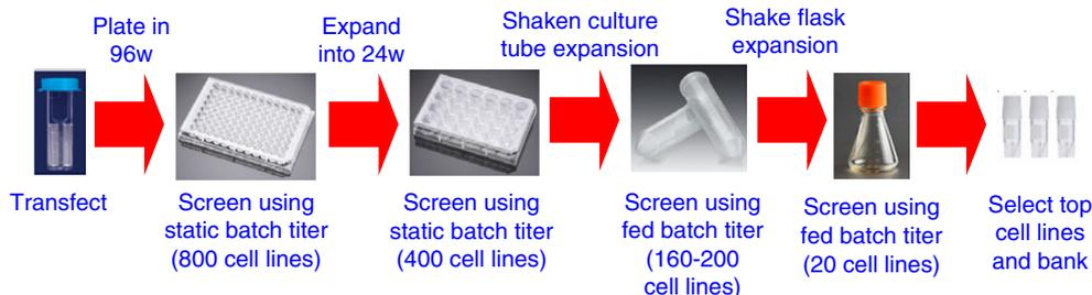
**Figure 1.** Overview of standard cell line development process. Initial screens were 96 and 24 shallow well (96w and 24w) static batch titers and shaken culture tubes. Final shake flask screen identified top six cell lines for banking.
