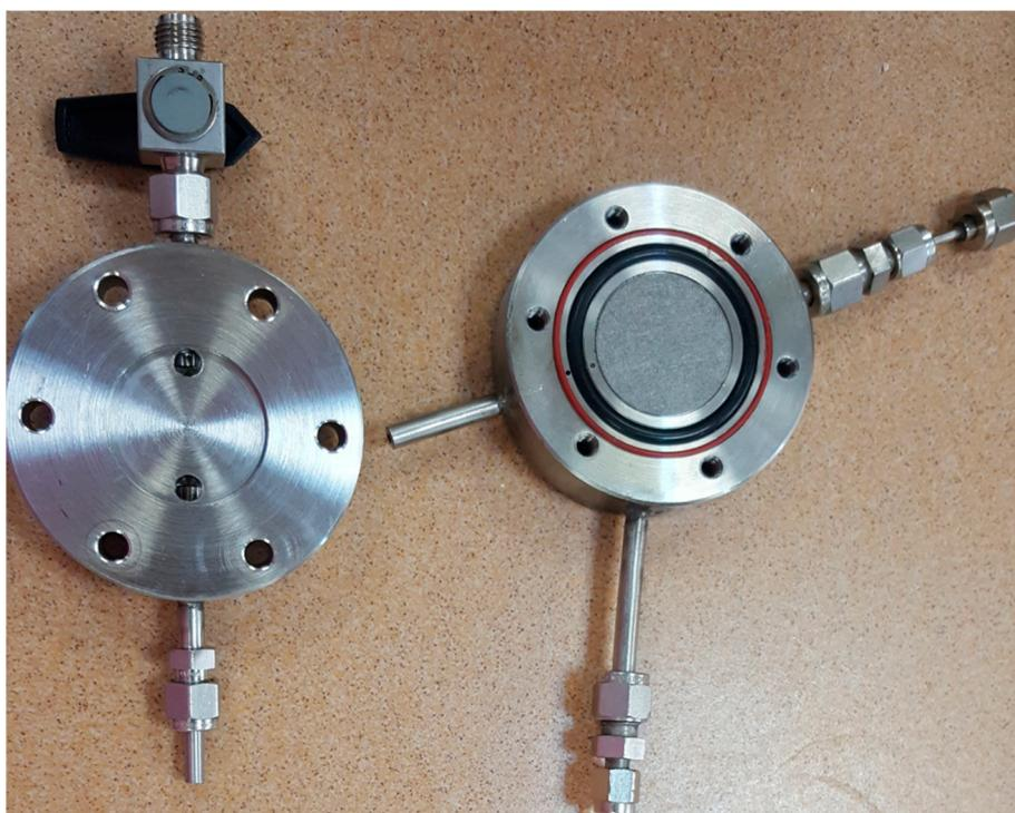
**Figure 1.** Membrane cell set-up.
