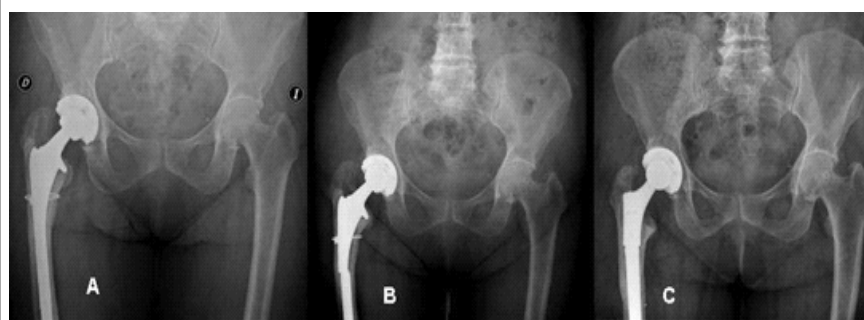
Figure 2: Radiological evolution after revision surgery; X-ray AP views: 2.A) 1 year after primary hip revision; 2.B) 37 Months after revision surgery; the femoral stem fractured at the junction between the proximal loose part and distally well-fixed zone and 2.C) 1 year after revision of the fatigued femoral stem
