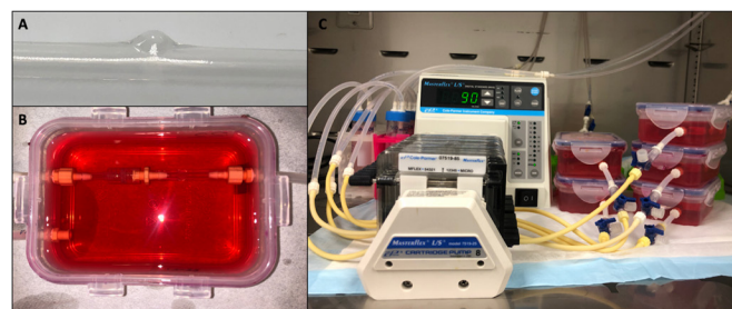
Figure 1 Silicone aneurysm tubes and bioreactor system configuration. Silicone aneurysm tubes were 43 mm in length, with 4.0 mm internal diameter, and incorporated aneurysms with a 2.4 mm neck and 3.1 mm height (A). Silicone aneurysm tubes were coated with fibronectin then placed in individual bioreactor chambers prior to cell deposition (B). Individual bioreactor systems were connected to media reservoirs, placed on peristaltic pumps, and run at 37°C and 5% CO 2 , before and after cell deposition (C).
