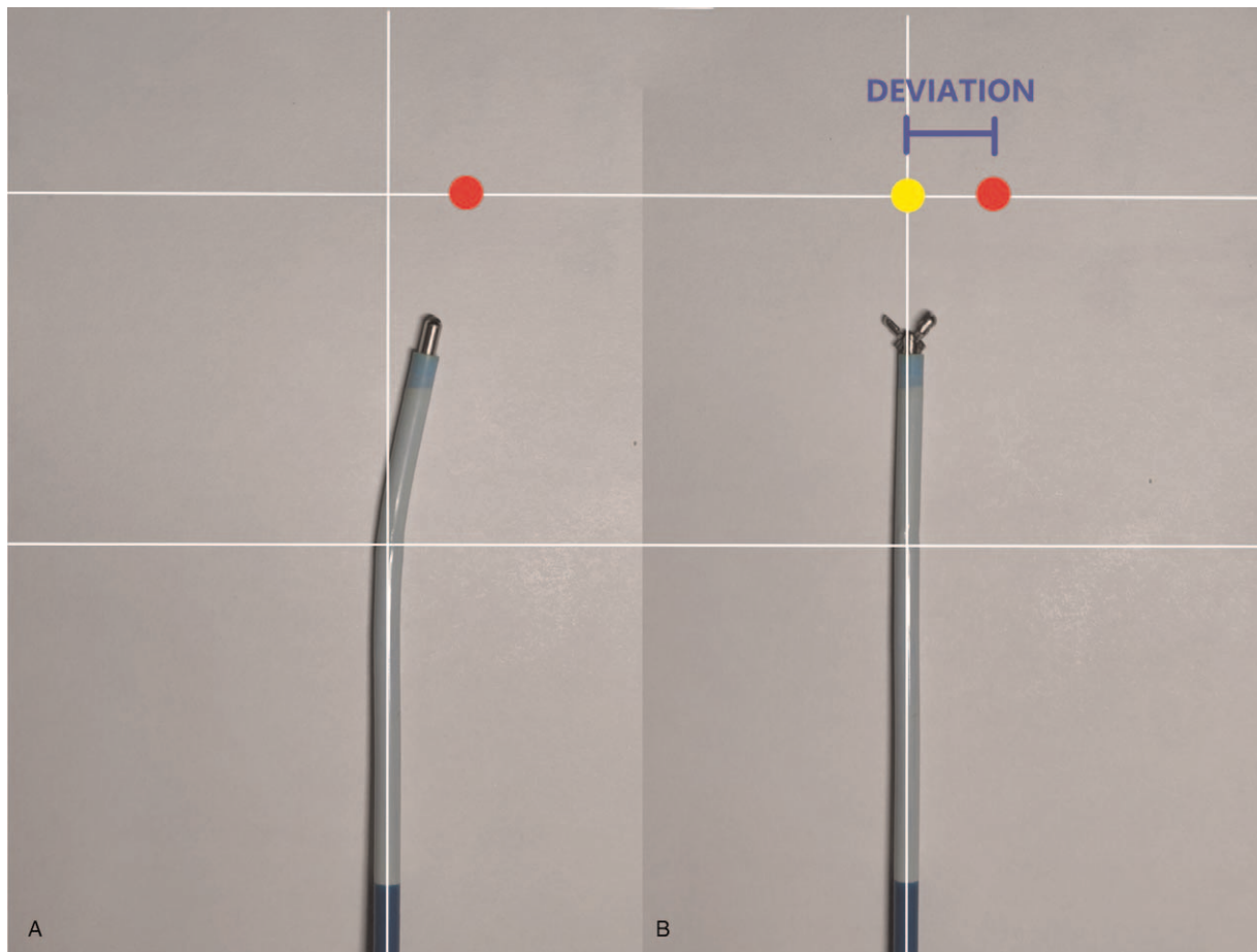
Figure 3. Deviation between sensor head and biopsy tool. A, the simulated sensor head reaches the lesion in tension-free conditions; B, the simulated angle change when the sensor head is withdrawn and the biopsy tool is outstretched.
