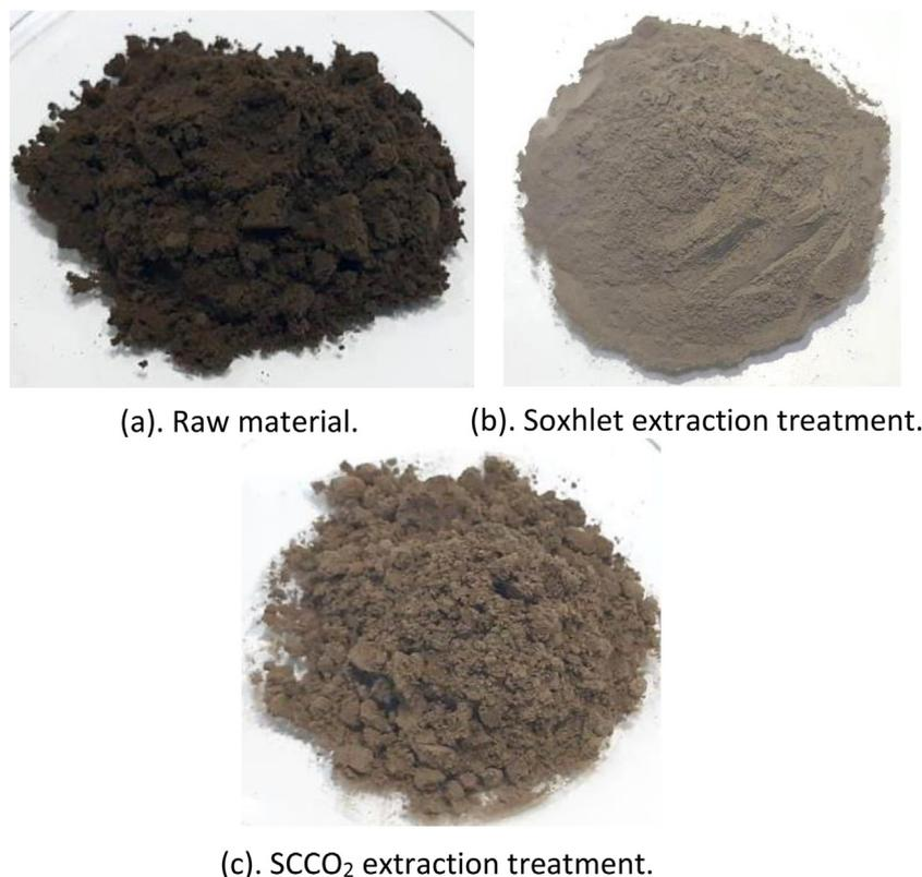
Figure 2. Photographs of SBE matrix (a) before and (b-c) after treatments.
