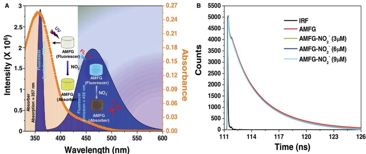
Fig. 4 (A) Absorbance and emission spectra of AMFG showing significant spectral overlap. (B) Fluorescence lifetime decay curves of AMFG in the absence and presence of different concentrations of  $\text{NO}_2^-$ .
