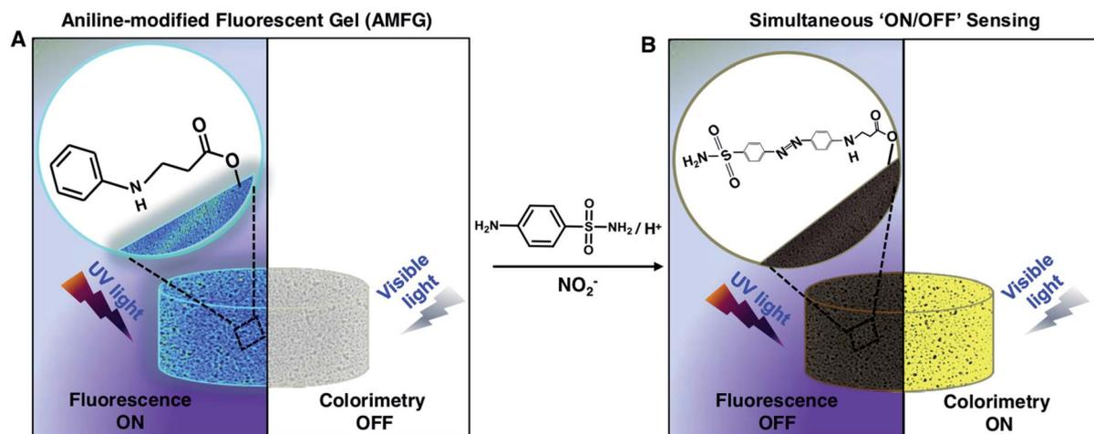
**Scheme 2** A schematic representation of AMFG under visible and UV light (365 nm) before (A) and after (B) the parallel 'ON/OFF' sensing of  $\text{NO}_2^-$  in the presence of sulfanilamide. The formation of the diazo dye in the porous gel led to a simultaneous change in color (white to yellow; colorimetric mode is 'ON') and the fluorescence signal (quenched from blue to dark; fluorometric mode is 'OFF') under visible light and UV light, respectively.
