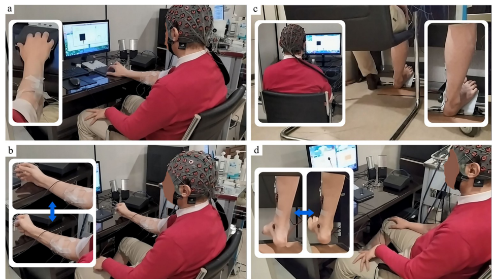
Fig 2. The experimental setup of the study. Four completed tasks, subjects, channels, and setup are presented in the picture. A) In task 1 as a static task; subjects did the task with the middle finger and held the output force in a specific range. B) In task 2 as a dynamic task; subjects opened and closed their hand with normal voluntary speed. C) Task 3 is static; the subjects held the pedal to generate the output force in the considered range. D) Task 4 as a dynamic task, subjects did the dorsiflexion and plantar flexion with normal voluntary speed. For all the tasks, subjects saw the monitor to do the task based on the timeline shown on screen.
