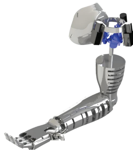
FIGURE 9: A CAD design of the prosthetic upper limb.
