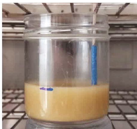
Fig. 1. The placement of the thermocouple inside the sample.
