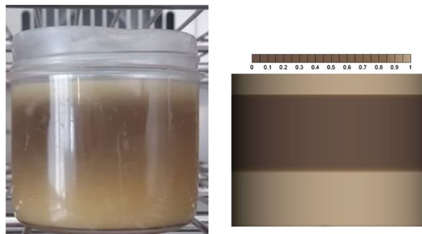
Fig. 8. Comparison of gelation propagation of numerical (right image) and experimental (left image) method after 60 min. The fraction of phase 2 (gel) is plotted on the right image.
