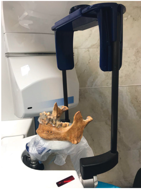
FIGURE 1: Teeth mounted on a dried mandible bone in the CBCT unit.
