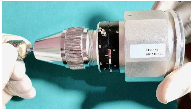
Figure 4. Extraction of implants from the bone using the torque calibrator (Sundoo STK-150cN.m Gauge).
