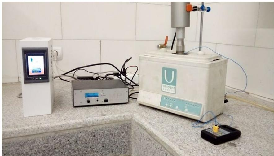
**FIGURE 2** Ultrasound-assisted extraction system schematic
