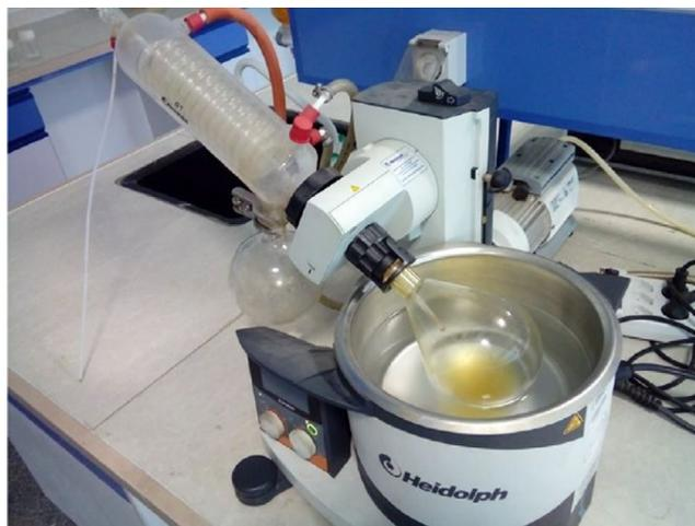
**FIGURE 3** Heidolph (Beals Hei-VAP Value) rotary evaporator
