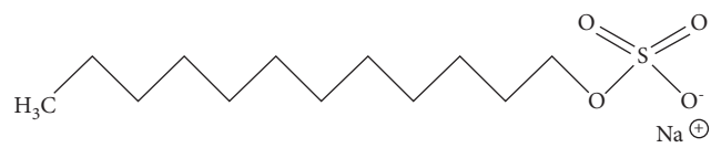
FIGURE 2: Chemical structure of sodium dodecyl sulfate.
