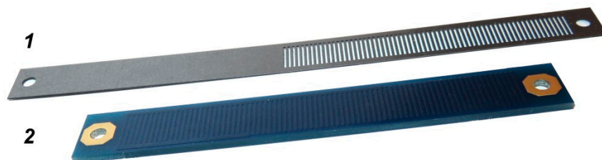
Figure 6. Measurement scales used for the simulation and the characterization of the microsystem. 1—transformer steel laser cut scale with 0.35 mm thickness; 2—PCB scale with 35 \mu m copper thickness. Full and void parts of the scale are each 0.5 mm wide, resulting in a scale period of 1 mm.
