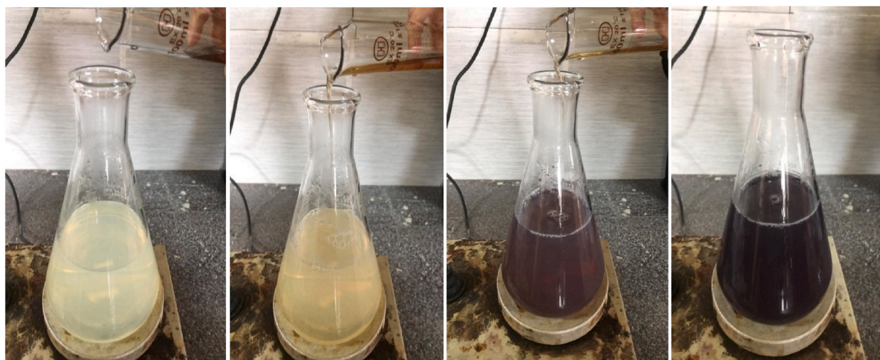
Fig. 2. Colour change in synthesis of AuNPs with the passage of time.
