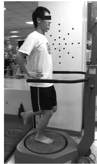
Fig. 2. Photograph of a subject demonstrating the measurement of dynamic balance using the Biodex Stability System.
