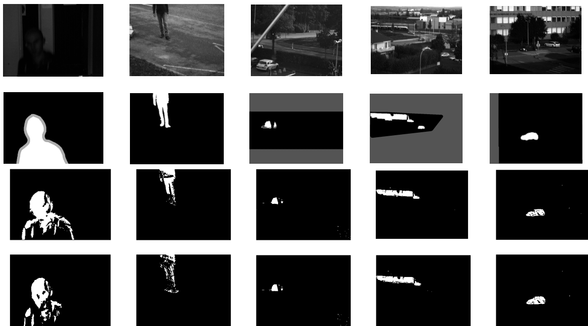
Figure 4. Background subtraction results on five videos. The top row is original multispectral sequences. The second row is the corresponding ground truth. The third and fourth are the results obtained by the respective best combination of multispectral and RGB sequences.
