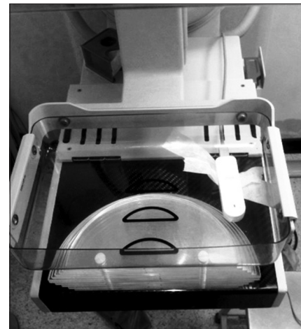
Figure 1: Experimental set up for measurement of breast entrance exposure in mammography phantom
