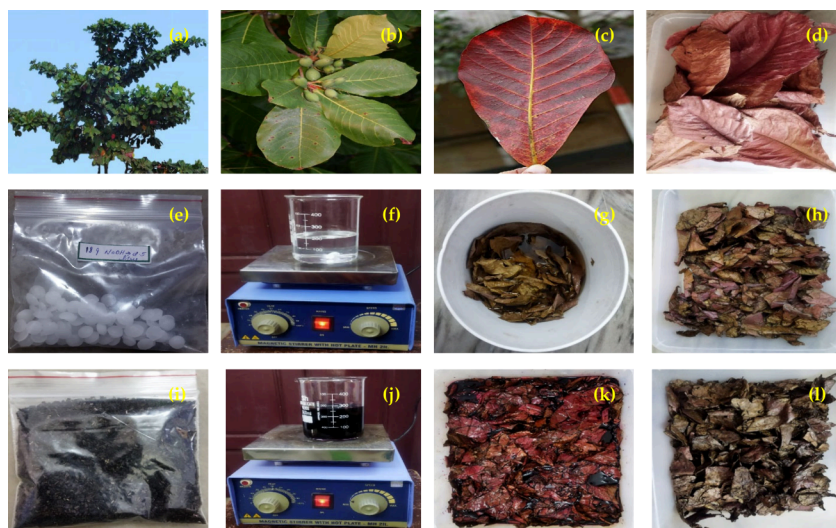
Figure 1. Terminalia catappa leaf fibers: (a) Tc tree, (b) Tc leaves, (c) dried Tc leaf, (d) dried Tc foliage, (e) NaOH pellets, (f) NaOH solution, (g) alkali treatment on Tc leaves, (h) dried NaOH treated Tc leaves, (i) potassium permanganate salt, (j) permanganate solution, (k) permanganate treatment on Tc leaves, (l) dried \text{KMnO}_4 treated Tc leaves.
