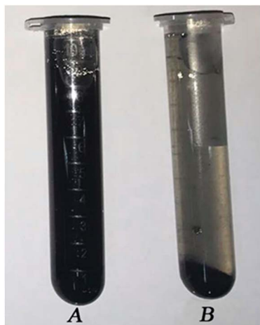
Fig. 8 The photographs of the GNPs dispersion which were allowed to stand for one month: (A) modified GNPs and (B) pure GNPs.
