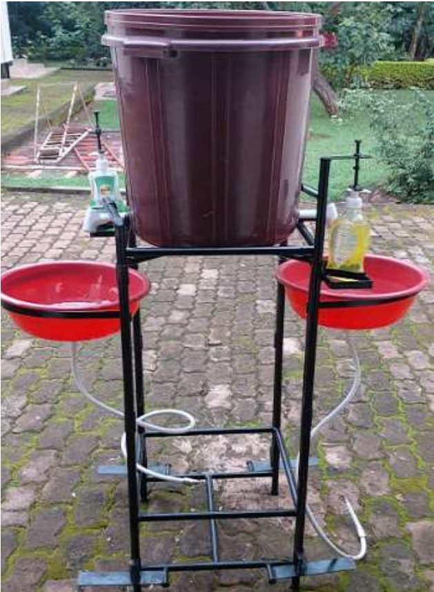
Figure 2: a hand-washing device that uses a foot pump for dispensing both the water and liquid soap donated by IPH-KCMUCo to the central market in Moshi municipality and ward executive office
