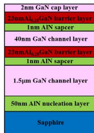
Figure 3. Diagram of the double channel epitaxial layer.
