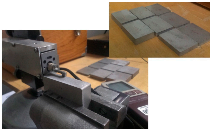
Figure 1. The sample to measure surface roughness with the measuring equipment.
