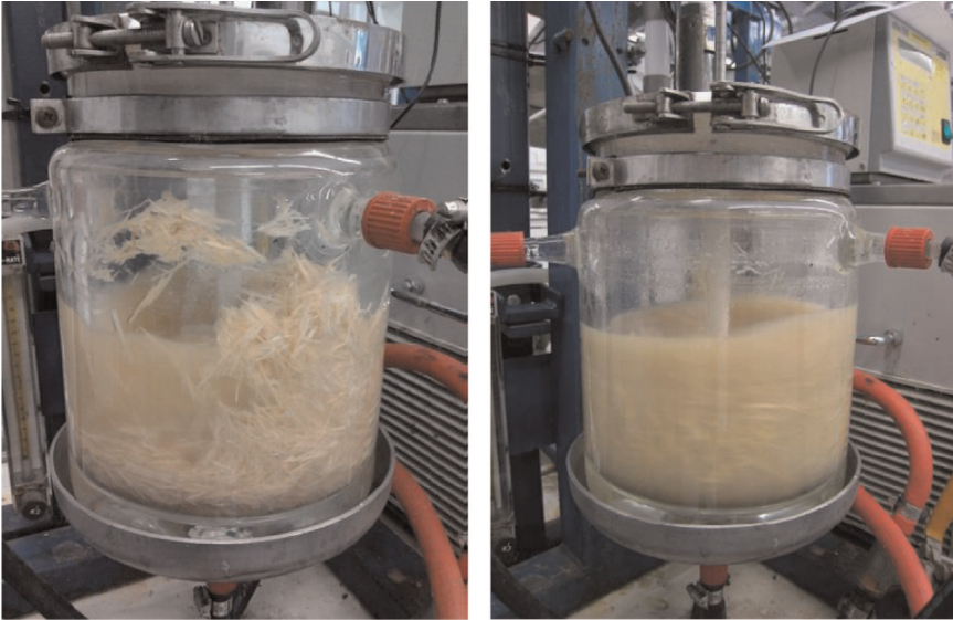
Fig. 3. Enzyme hydrolysis start (above) and stop (below). Sample: chipped softwood of pine. Volume of the bioreactor: 3.5 L; Solution: 2 L water; Solid/liquid ratio 40; Mixing rate 250 rpm; Temperature 30 °C; Pressure 2 bar. (Photographs by Päivi Riikonen).
