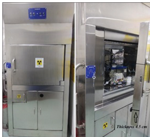
Figure 1: Hot cell to house ^{68}\text{Ga} iQS-TS Synthesis module, ITG, Germany
