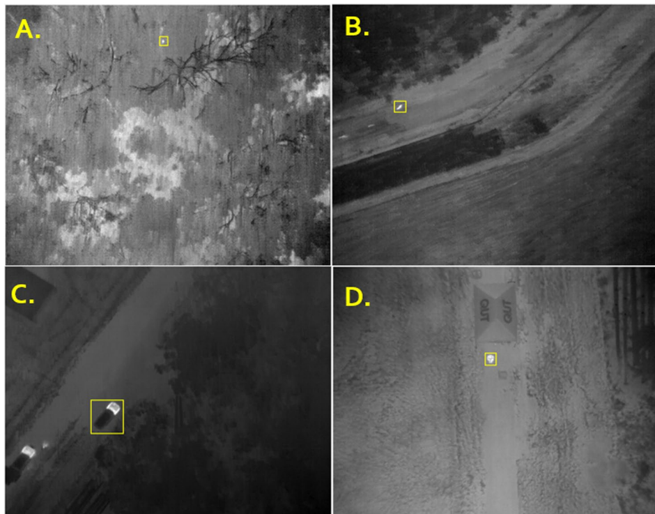
Figure 3. Objects automatically detected in RPAS-derived thermal imaging: (A) Candidate koala signature, (B) Kangaroo, (C) Car, (D) Human.
