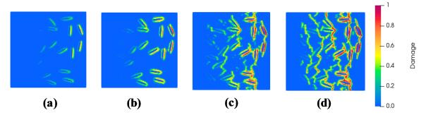
**Figure 5.** Progressive damage observed in iron powder (10%) modified HCP corresponding to applied tensile strains of (a) 24  $\mu\varepsilon$ , (b) 78  $\mu\varepsilon$ , (c) 121  $\mu\varepsilon$  and (d) 130  $\mu\varepsilon$ .
