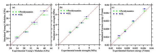
**Figure 9.** Correlation between experimental and simulated (peridynamics and finite element (FE) approach) (a) Young's modulus and (b) tensile strengths and (c) fracture energy of mortars with various dosage of waste iron powder.
