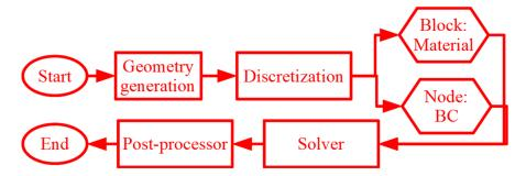
Figure 1. A schematic framework for peridynamics-based micromechanical modeling.
