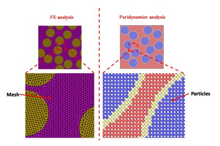
**Figure 3.** Sample mortar unit cell to describe the mesh-free approach in peridynamics as contrasted with the finite element (FE) mesh.
