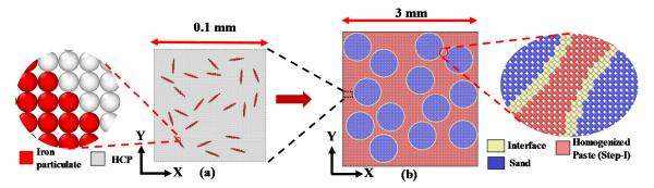
**Figure 4.** Interactive length scales: (a) Step I: 10% iron powder dispersed in hardened cement paste (HCP) matrix at micro-scale; (b) Step II: sand embedded in homogenized iron powder- HCP at meso-scale (the homogenized material from (a) serves as matrix for (b)).
