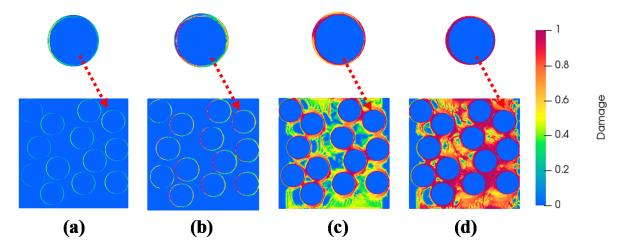
**Figure 7.** Progressive damage (interface/matrix) observed in iron powder (10%) modified mortar corresponding to applied tensile strains of (**a**) 52  $\mu\varepsilon$ , (**b**) 105  $\mu\varepsilon$ , (**c**) 153  $\mu\varepsilon$  and (**d**) 208  $\mu\varepsilon$  (the interface damage is highlighted in zoomed pictures).
