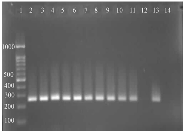
Fig. 1 The products of PCR electrophoresed on 1.5% agarose. For proper dilutions, no bands were observed during the electrophoresis. Line 1: Ladder 100 bp, Line 2–11: Improper dilutions, Line 12: Proper dilution: Streptavidin (1:256), Ab monoclonal (1:32,000), Line 13: Improper dilutions, Line 14: Negative control
