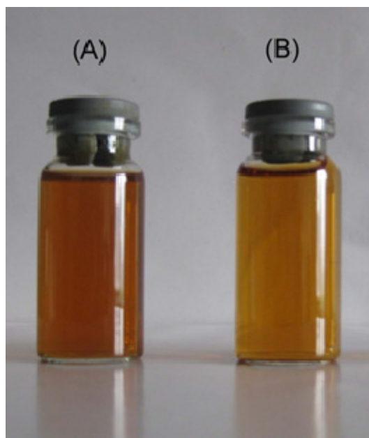
Figure 2. Appearance of (A) raw; (B) filtered by 0.2 \mu\text{m} \text{ZrO}_2 membrane.
