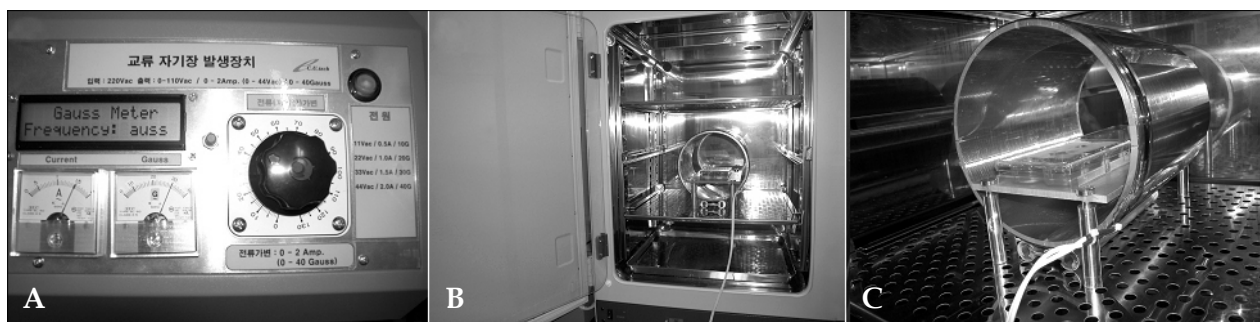
Fig. 1. EMF exposure system. (A) Control part. (B) Placement of the system and position of the sample in a cell culture incubator. (C) Magnified view of the experimental setup.
