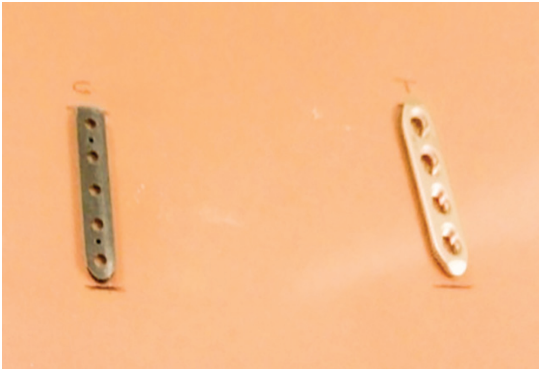
Fig.1 Photo of setup #1, carbon plate on the left and titanium alloy on the right.
