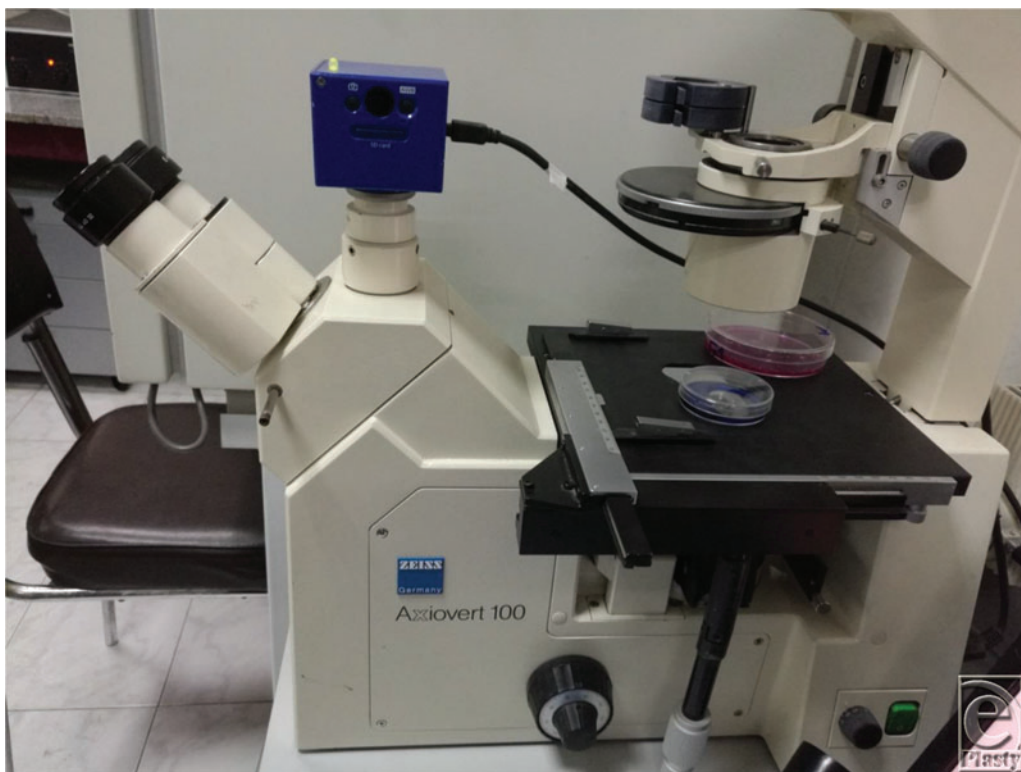
Figure 2. Inverted microscope (Axiovert 100; Zeiss, Jena, Germany).
