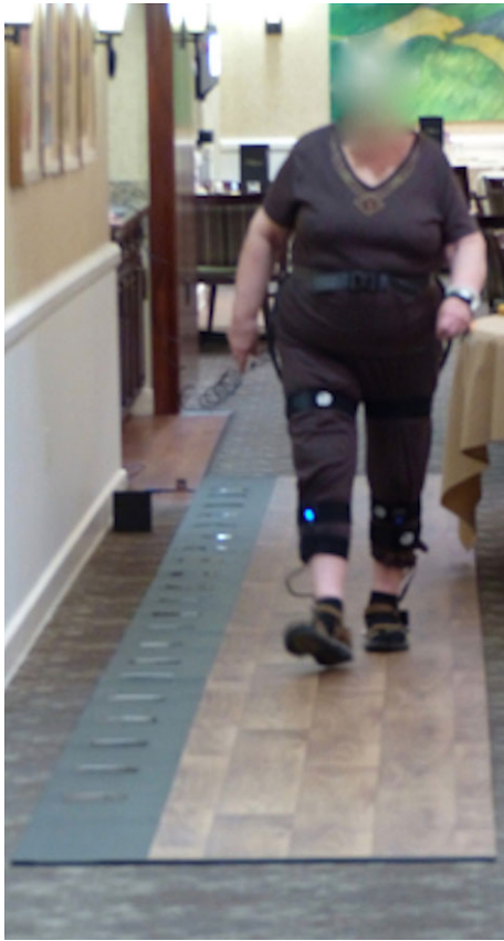
Fig. 4. Electronic Gait Mat. Spatiotemporal Gait Parameter Collection for Subject Walking on Electronic Gait Mat.
