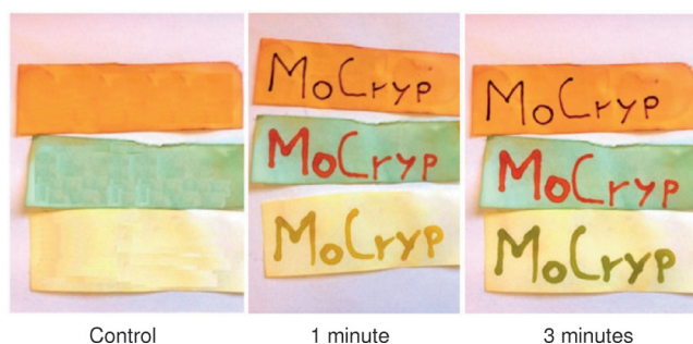
Figure 9. Writing with trichocyanines generated in situ. Left: the control shows filter paper strips dipped into three different aldehyde solutions in methanolic p -toluenesulfonic acid (top: 4-dimethylaminocinnamaldehyde, middle: ferulic aldehyde, bottom: 4-dimethylaminobenzaldehyde). Middle: image taken immediately after writing on the stripes with a methanol solution of 3-phenyl-2 H -1,4-benzothiazine. Right: image 3 min after writing.
