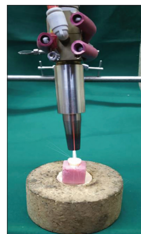
Figure 1: Nonthermal atmospheric plasma application on the rewetted surface of a specimen
